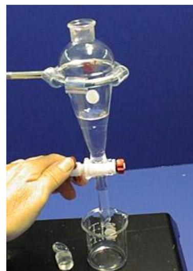
Carefully open the stopcock and allow the lower layer to drain into the flask. Drain just to the point that the upper liquid barely reaches the stopcock
