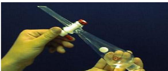
Then, point the stem up and slowly open the stopcock to release excess pressure. Close the stopcock. Repeat this procedure until only a small amount of pressure is released when it is vented
