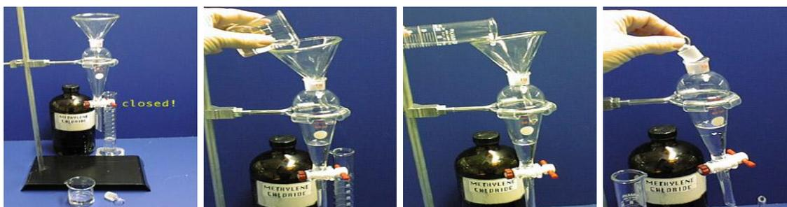
1. Support the separatory funnel in a ring on a ringstand. Make sure stopcock is closed
