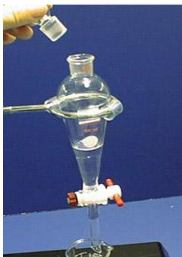
While waiting, remove the stopper and place a beaker or flask under the sep funnel.
