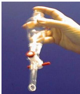
Now, shake the funnel vigorously for a few seconds. Release the pressure, then again shake vigorously. About 30 sec total vigorous shaking is usually sufficient to allow solutes to come to equilibrium between the two solvents.
