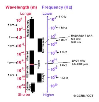
For most purposes, the **ultraviolet or UV** portion of the spectrum has the shortest wavelengths which are practical for remote sensing. This radiation is just beyond the violet portion of the visible wavelengths, hence its name. Some Earth surface materials, primarily rocks and minerals,fluoresce or emit visible light when illuminated by UV radiation.
