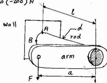
$$S_f = C_{load} C_{size} C_{surf} C_{temp} C_{reliab} S_f' \\ = (1) (1) (0.898) (1) (0.753) 130 = 87.905 \text{ MPa}$$
